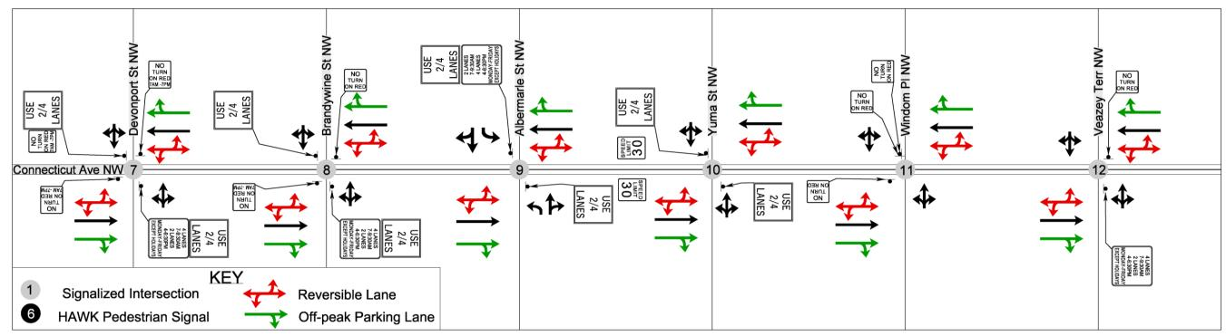
Figure 9: Traffic Control, Operational Signage, Parking, and Lane Geometry from Devonport Street NW to Veazey Terrace NW
