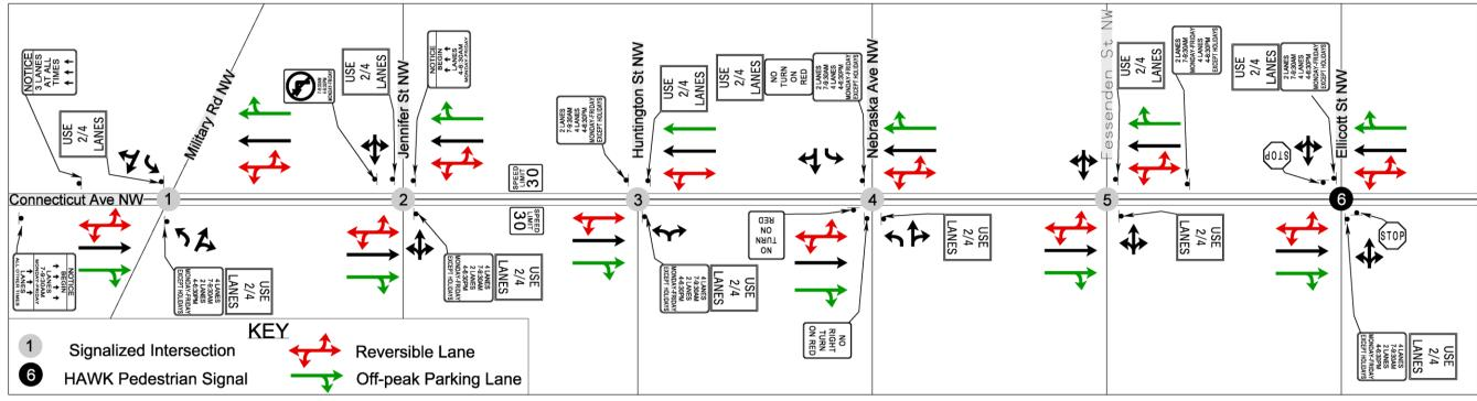
Figure 8: Traffic Control, Operational Signage, Parking, and Lane Geometry from Military Road NW to Ellicott Street NW
